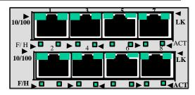
default setting) are independently N-way auto-negotiating, and auto-crossover(MDIX) for operation at 10 or 100Mb speed in full- or half-duplex mode, i.e., each independently selects a mode and speed to match the device at the other end of the twisted pair cable.
